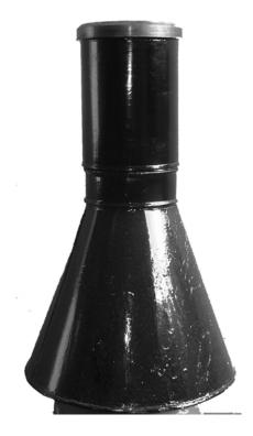
The Non-recording Rain Gauge is used to take daily measurements of rainfall. It has been designed by the British Meteorological Office. Illustrated rain gauge is made of gauge 24 G.I sheet locally, according to the Department of Meteorology specifications painted with anti-corrosive black color. This version of conical design helps to sit firmly on a leveled floor (Cylindrical shape rain gauge can be easily rolling on the floor)
